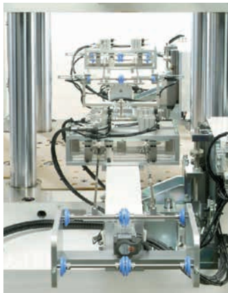
View from hoop material ejection side (side view of the molding machine)
