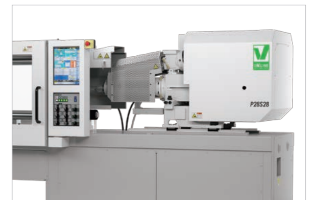
Example of safety standard compliance: Purge cover, plasticization cylinder cover
