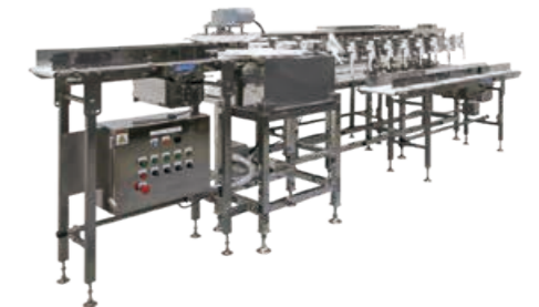
Upward-facing tray de-breading machine: A machine that removes frozen foods, including toppings, from their freezing containers. Removing the product face-up eliminates topping loss, reduces labor requirements, and mitigates the risk of foreign matter contamination.
