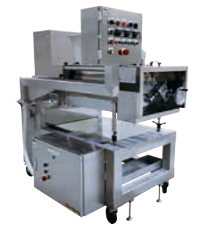
Three-roll sheeter: A machine that forms elastic and viscous doughs (such as high-hydration noodle dough or pastry dough) into sheets by gently pressing them through three rollers
