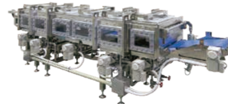
Continuous vacuum cooling equipment that alternately vacuum-cools two parallel cooling chambers. By cooling food in a short time, it suppresses bacterial growth and deterioration of taste.
