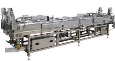
Continuous vacuum cooling equipment. By alternating vacuum cooling between two chambers, the equipment enables continuous processing while rapidly cooling food products to suppress bacterial growth and maintain product quality and flavor.
