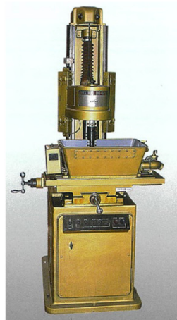
Japaxtron D3 (1954), First practical Die-sinker EDM in Japan
