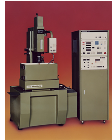
22 NC 8000 (1980), the oldest existing Die-sinker EDM equipped with a microcomputer NC
