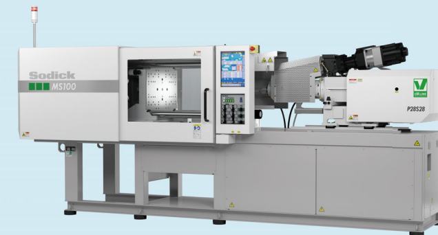
INFILT-V®, inert gas dissolution injection molding system Recipient of the 18th (2021) Super Monozukuri Parts Award, Environment, resource- and energy-related parts awards
