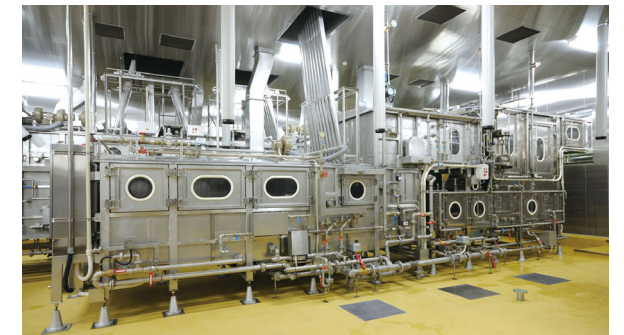
Boiling machine equipped with CIP automated cleaning
