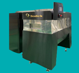
High-temperature pressure sterilizer (cooked rice, boxed meals, precooked side dishes) Container and rice are sterilized simultaneously and quickly using saturation vapor heated to more than 100°C
