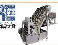
It was evaluated that the addition and stirring process of seasoning liquid such as sauce, etc., in the production of cooked noodles, which used to be done manually in the past, was made unmanned to reduce the risk of contamination by bacteria and foreign substances, to reduce food loss by extending freshness, to reduce costs by saving labor, and to realize advanced cleaning performance.
