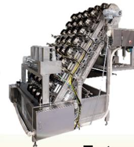
It was evaluated that the addition and stirring process of seasoning liquid such as sauce, etc., in the production of cooked noodles, which used to be done manually in the past, was made unmanned to reduce the risk of contamination by bacteria and foreign substances, to reduce food loss by extending freshness, to reduce costs by saving labor, and to realize advanced cleaning performance.
