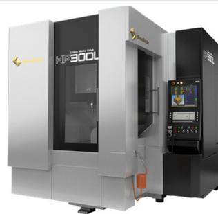
Revamped linear motor-driven machining center
