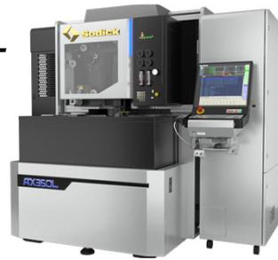
Super-precision wire-cut EDM that meets the demand for long-time stable processing and labor saving
