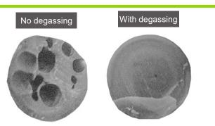
\*Cross-sectional comparison of metering materials Molding defects due to residual air (Left) Problem solved by this technology (Right) Our proprietary material feeder "Degassing-type Stuffer Box" has succeeded in eliminating most of the "air entering the material" that causes molding defects and material loss, and can improve the quality and productivity of rubber molding immediately.
