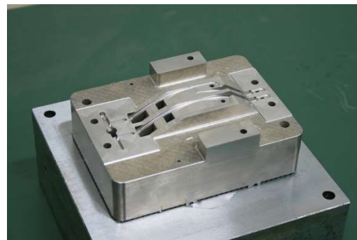
▲ A mold equipped with 3D cooling piping
