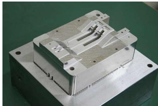
▲ A mold equipped with 3D cooling piping
