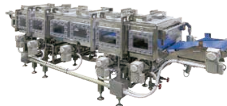
Continuous vacuum cooling equipment that alternately vacuum-cools two parallel cooling chambers. By cooling food in a short time, it suppresses bacterial growth and deterioration of taste.
