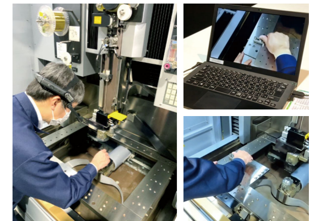
Use a wearable camera to take images of the entire machine, its surroundings, the operator's eye level, and the operator's hands, and display multiple images on the screen.
