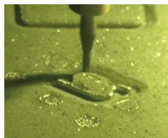
Cutting and machining process with a metal 3D printer
