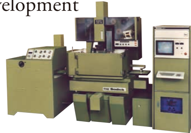
330W NC wire-cut EDM, which allows for 5-axis control
