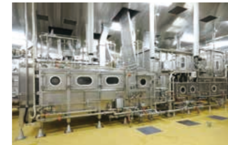
Boiling machine equipped with CIP automated cleaning
