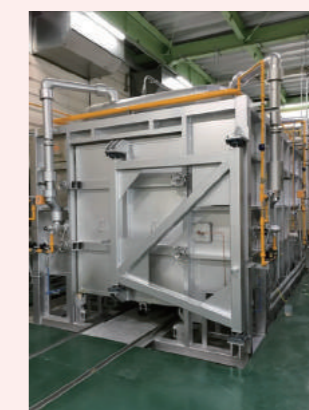
Ceramics kiln at the Kaga Plant
