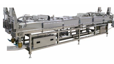
Continuous vacuum cooling equipment. By alternating vacuum cooling between two chambers, the equipment enables continuous processing while rapidly cooling food products to suppress bacterial growth and maintain product quality and flavor.
