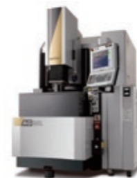
AG35L die-sinker EDM with linear motor drive
