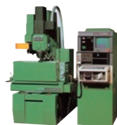
A3C-R NC die-sinker EDM
