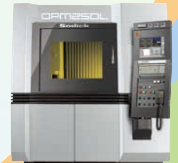
▲ Metal 3D printer "OPM250L"
