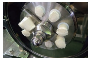
Extruder: Creating new textures by extruding in high vacuum
