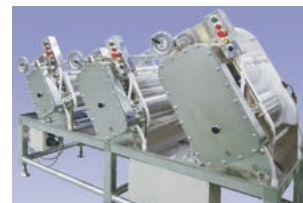
Continuous Noodle-sheet Press Roller: Noodle sheets are press rolled continuously and gradually so as not to impair the gluten structure of the noodle sheets
