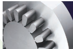
High-precision machining of motor core mold
