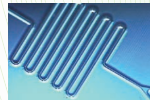
Ultra-fine flow channel machining (AZ275nano)
