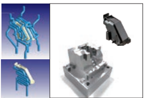
Enables innovative plastic-injection processes using molds with built-in conformal cooling pipes
