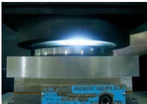
Machining of Speaker Mold by Die-Sinker EDM
