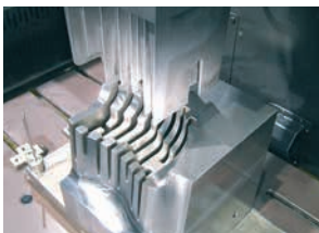
Electrode and Die after Die Sinking
