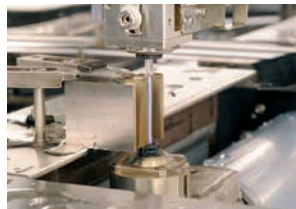
Cutting of Metal Piece with Wire-cut EDM
