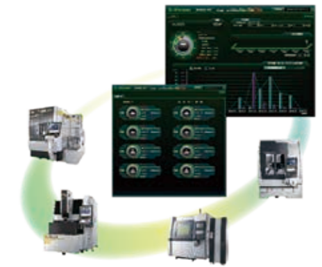
S-Viewer software that patrols each NC unit at fixed intervals to collect data
